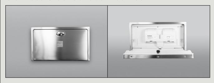
Colour Stainless Steel **Load Support** Up to 20kgs **Unit Weight** 23.9kg (net) Material 304 Stainless steel and polyethylene **Dimensions** 905W x 520H x 104D (closed) 495D mm (open) **Standards** Complys with EN12221 **Fixing** All fixings included + mounting template Warranty 12 Months **Product Code** SPBSSS40
